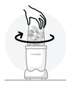
Turn the Cup upside down and place it onto the Motor Base, gently push and twist.
